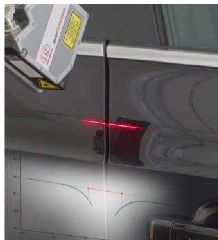
Gap and flushness measurement on bodywork parts
