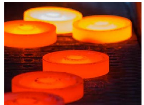
Temperature measurement in the metals industry Temperature monitoring in the cooling processes of forged parts using the CTLaser M1
