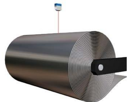
Measurement of coil diameters The quantity of steel wound on and off is monitored via the detection of the coil diameter using laser gauging sensors.
