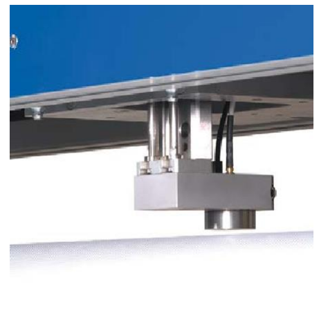
Non-contact, inline thickness measurement of plastic films
