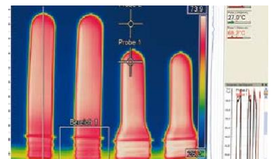
Thermal image shots of preforms in PET bottle production
