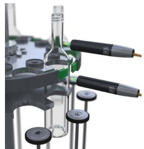
Measuring the thickness and roundness of bottles confocalDT 2422 is used to measure the thickness and roundness of glass bottles with two channels. Thickness calibration enables varying distances between the sensor and the bottles without influencing the measurement accuracy.
