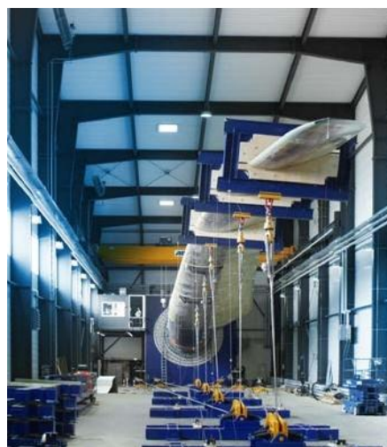
In test benches during load tests, several draw-wire sensors measure the deformation of rotor blades for wind turbines
