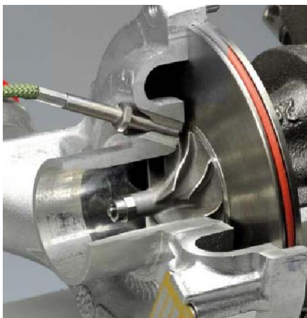
Rotational speed measurement of turbochargers
