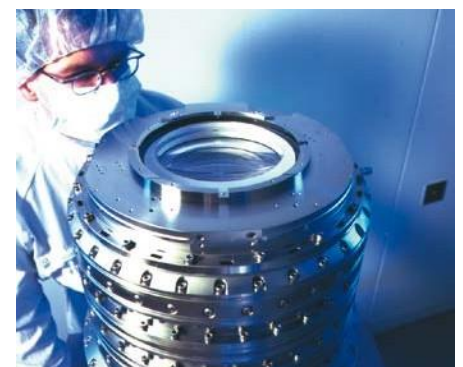
Non-contact, capacitive displacement sensors are used for nanometer adjustments of lenses in objectives for wafer exposures.
