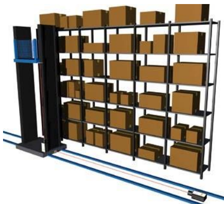
Position measurement in stacker cranes Fast response times combined with high measurement accuracy facilitate the exact positioning of stacker cranes.
