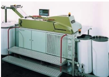
Example: machine monitoring Eddy current sensors monitor the fluctuating thickness of yarns in textile machines.
