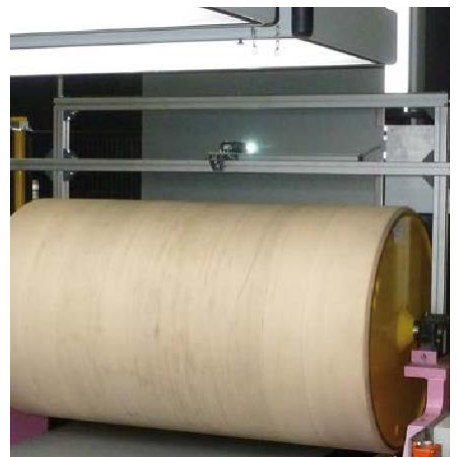
Color measurement of continuous strip coating such as aluminum, zinc and paper during production.
