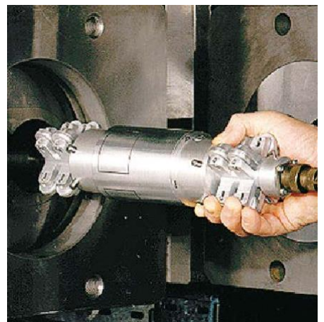
Inspection of inner diameter in extruder bores
