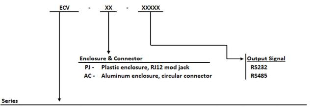
ECV - Electronic Compass with 3-axis magnetometer, 3-axis gyroscope, 2-axis tilt sensor & 3-axis accelerometer
